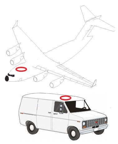
The graphic above shows examples of where the 42G1215A-XT-1 antenna may be located on an aircraft or vehicle (not to scale).
